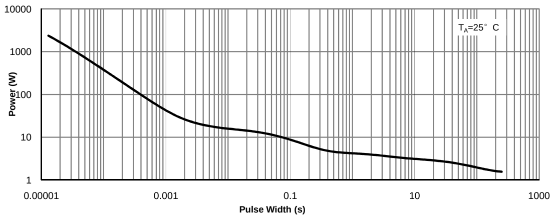
Figure 11: Single Pulse Power Rating Junction-to-Ambient (Note F)
